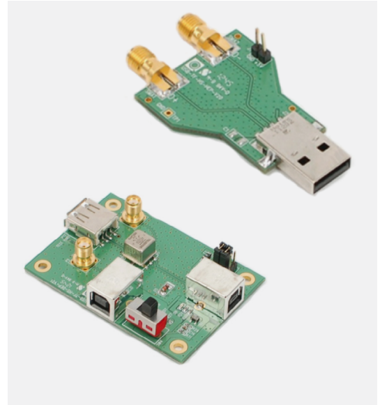
FIGURE 15. USB-IF USB2SIGQUAL Host (top) and Device (bottom) fixture set.
